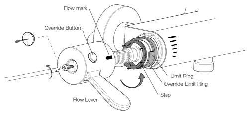
3. Remove the Flow Lever and adjust the Limit Ring so that it is aligned with the flow mark position. This will then set the maximum **Normal flow rate position** before the override button is depressed.
