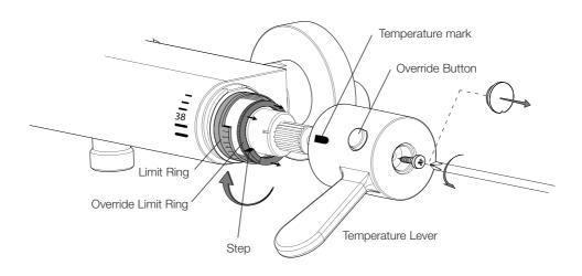
2. Turn the temperature lever to the fully cold position.
