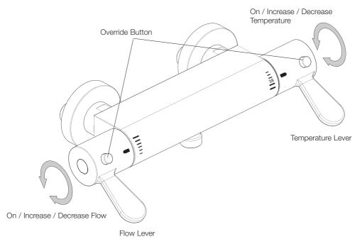
The maximum temperature is factory preset to approximately 41°C under ideal installation conditions at the factory.
